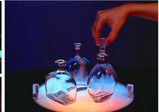
MusicBottles – opening and closing the lids starts and stops music of different styles (electromagnetic sensors)
