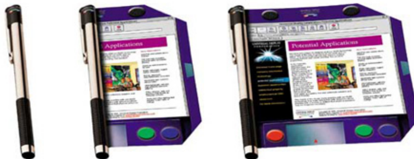
Universal Display Corp. Prototype of Pen with a built-in roll-up display (touch sensitive)
