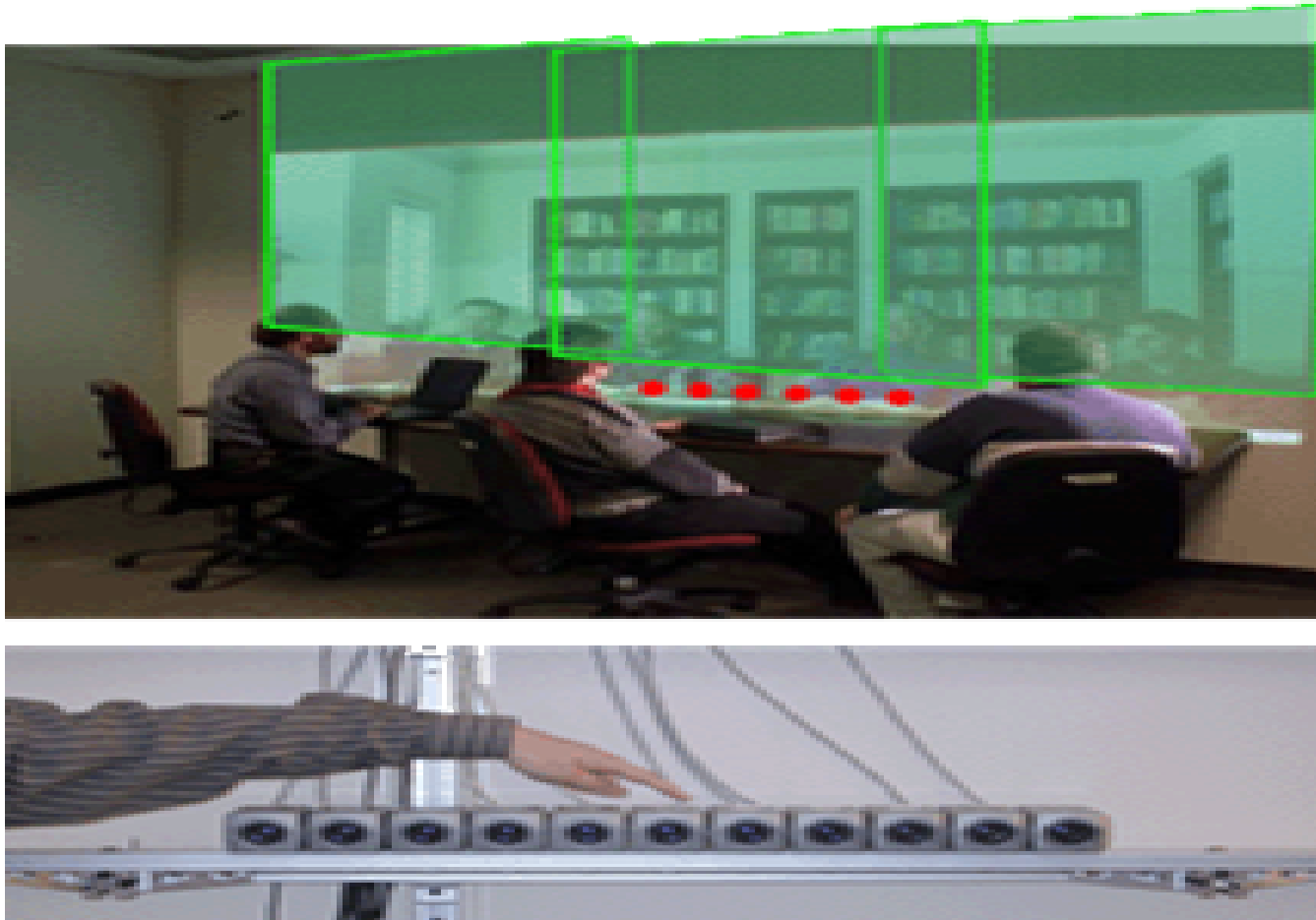
Line Light Field design: Abutted projector display with a dense horizontal camera array at table level and actual camera array implementation
