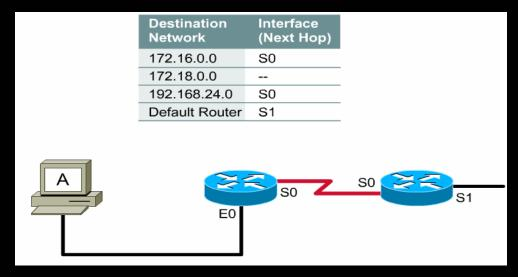
• The router accepts the packet on one interface, determines which path to use, and then proceeds to switch the packet.
